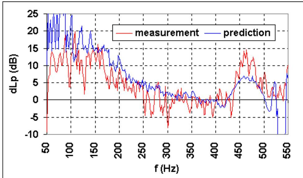
Fig. 22 Comparison of measured and predicted overall installation effect
