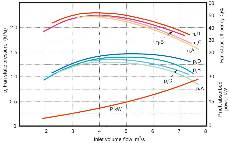
**Fig. 11 Typical performance curves for a forward curved centrifugal fan to different installation categories**
