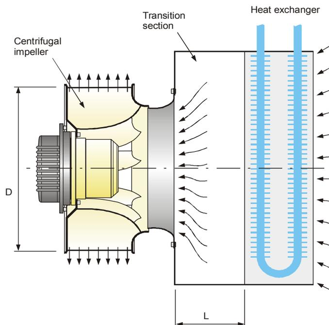
Fig. 29 Cooling unit set-up
