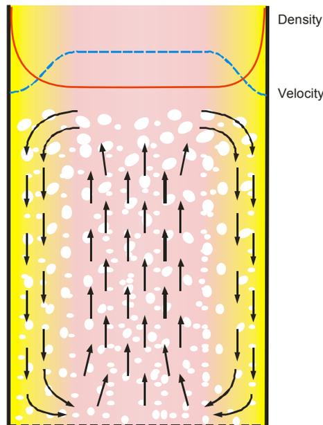
**Fig. A3. Typical particle motion inside the circulating fluidized bed reactor. The solid density increases near to the walls because the gas velocity is lower. Part of the particles combine together to form particle agglomerates known as clusters. These clusters are falling downwards and form internal material circulation inside the reactor or combustion chamber. (Redrawn from Raiko et al. 1995.)**
