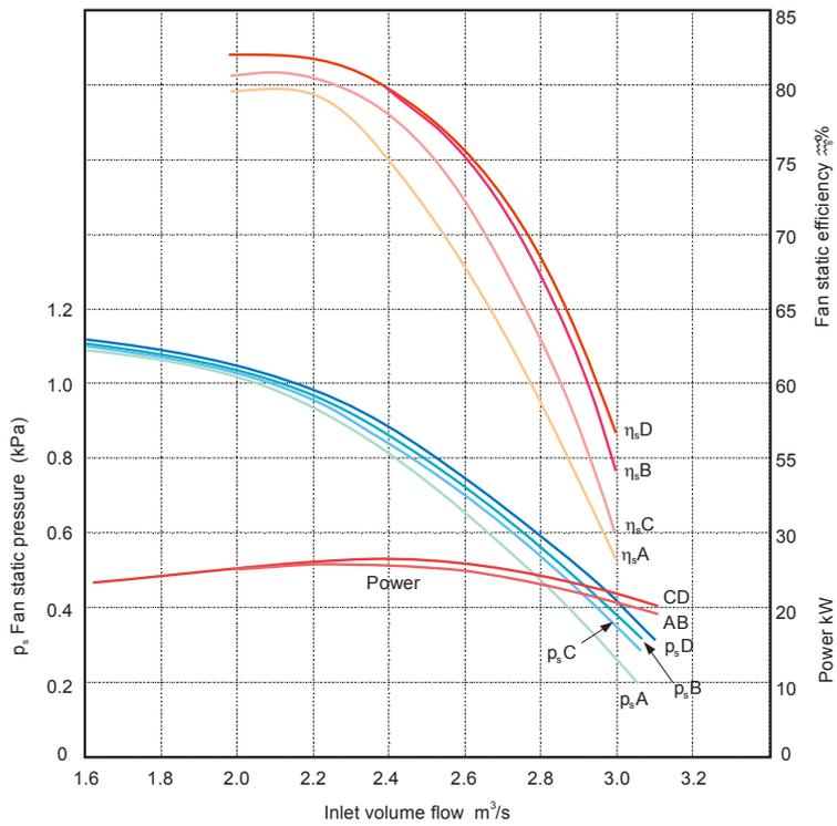
**Fig. 12 Typical performance curves for a backward inclined centrifugal fan to different installation categories**
