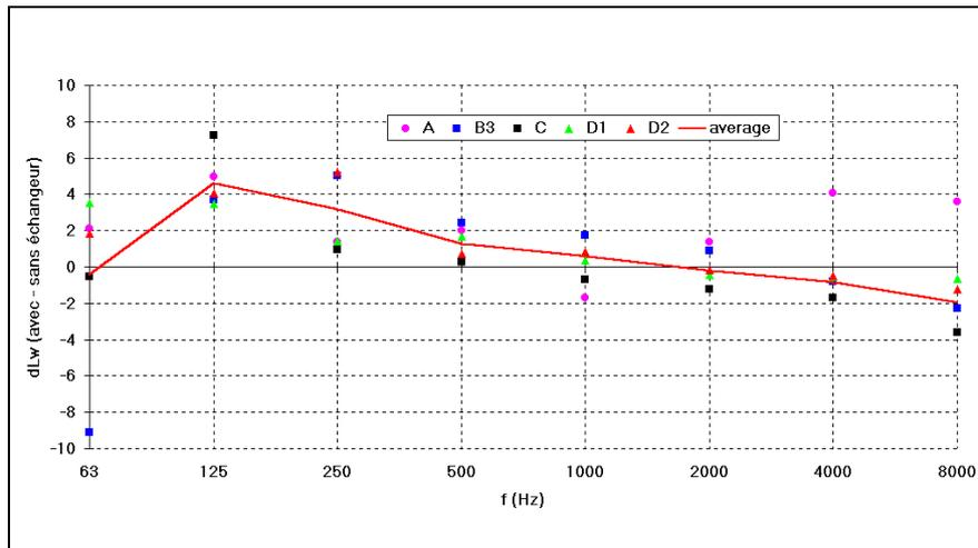
**Fig. 25 Exchanger at the fan inlet**  $dL_W \text{ (dB)} = L_W \text{ with exchanger} - L_W \text{ without exchanger}$
