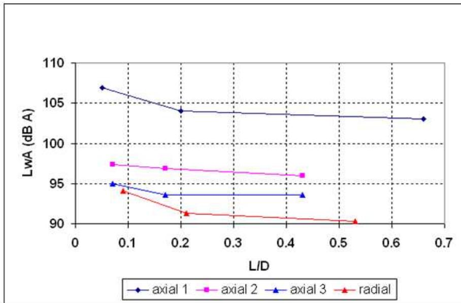
Fig. 28 Influence of the distance between the fan and the radiator on the A-weighted sound power level at constant flow  $Q_v = 3 \text{ m}^3/\text{s}$
