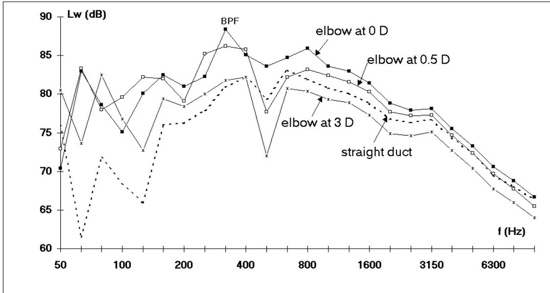
**Fig. 18b Comparison of fan inlet sound power spectra for different inlet configurations**
