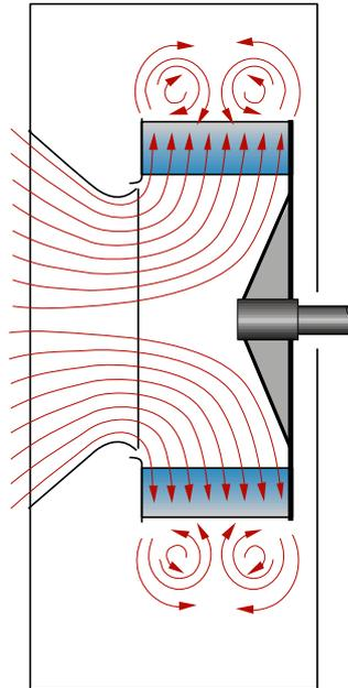
**Fig. 15 Forward curved centrifugal fan showing contra swirl at the outlet from the impeller**
