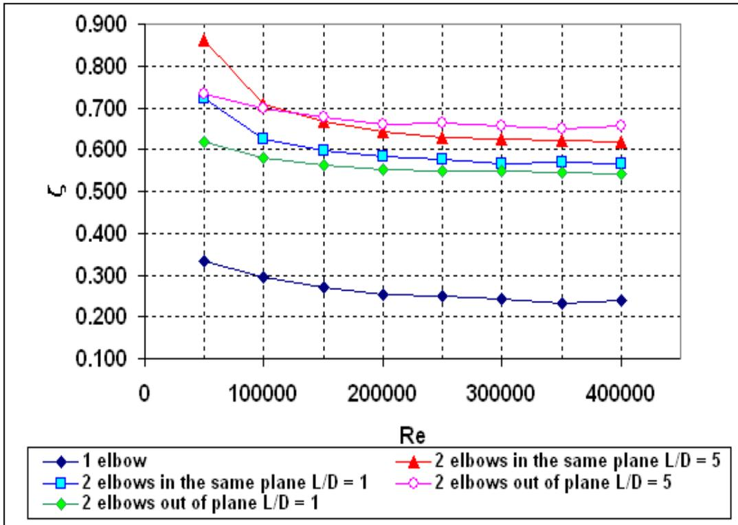
Fig. 7 Energy loss coefficient of 90° elbows (lobster backed bends)
