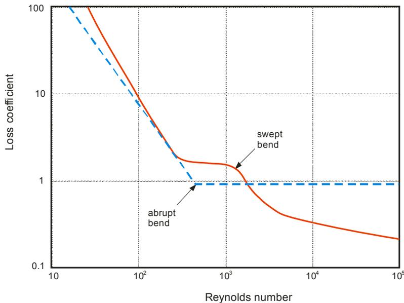
Fig. 4: Bend loss coefficients for transitional flows
