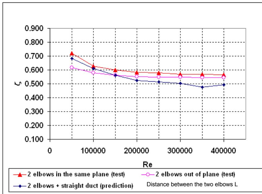
Fig. 9 Energy loss coefficient of 2 elbows separated by a duct  $L/D = 1$
