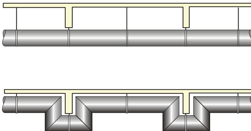
**Fig. 16 Ventilation duct running along the ceiling of an industrial building**
