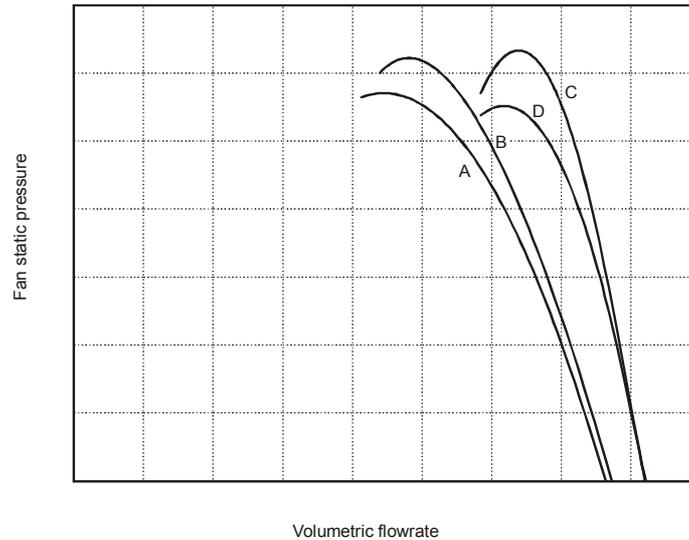
**Fig. 13 Typical performance curves for a tube axial fan to different installation categories**
