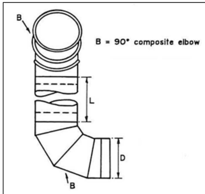
Two 90° composite elbows out of plane dia. 250 mm
