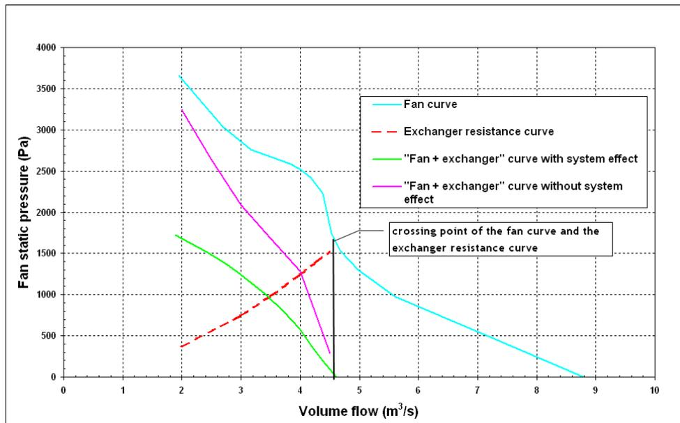
**Fig. 23 Evaluation of installation effect on fan performance**
