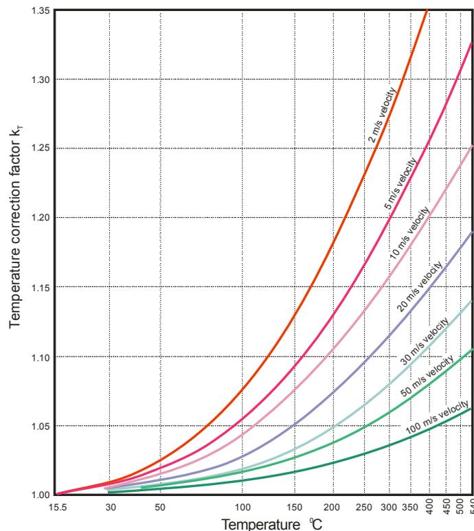
**Fig. 5 Temperature correction chart for duct friction due to viscosity and Reynolds Number changes**
