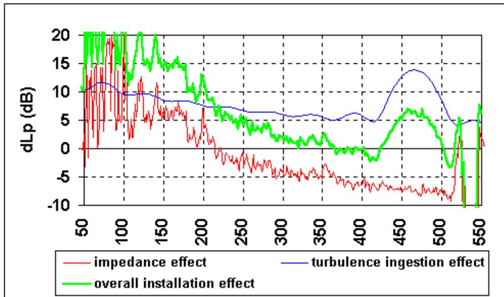
**Fig. 21 Prediction of installation effect ( $dLp = Lp_{with\ box} - Lp_{reference}$ )**
