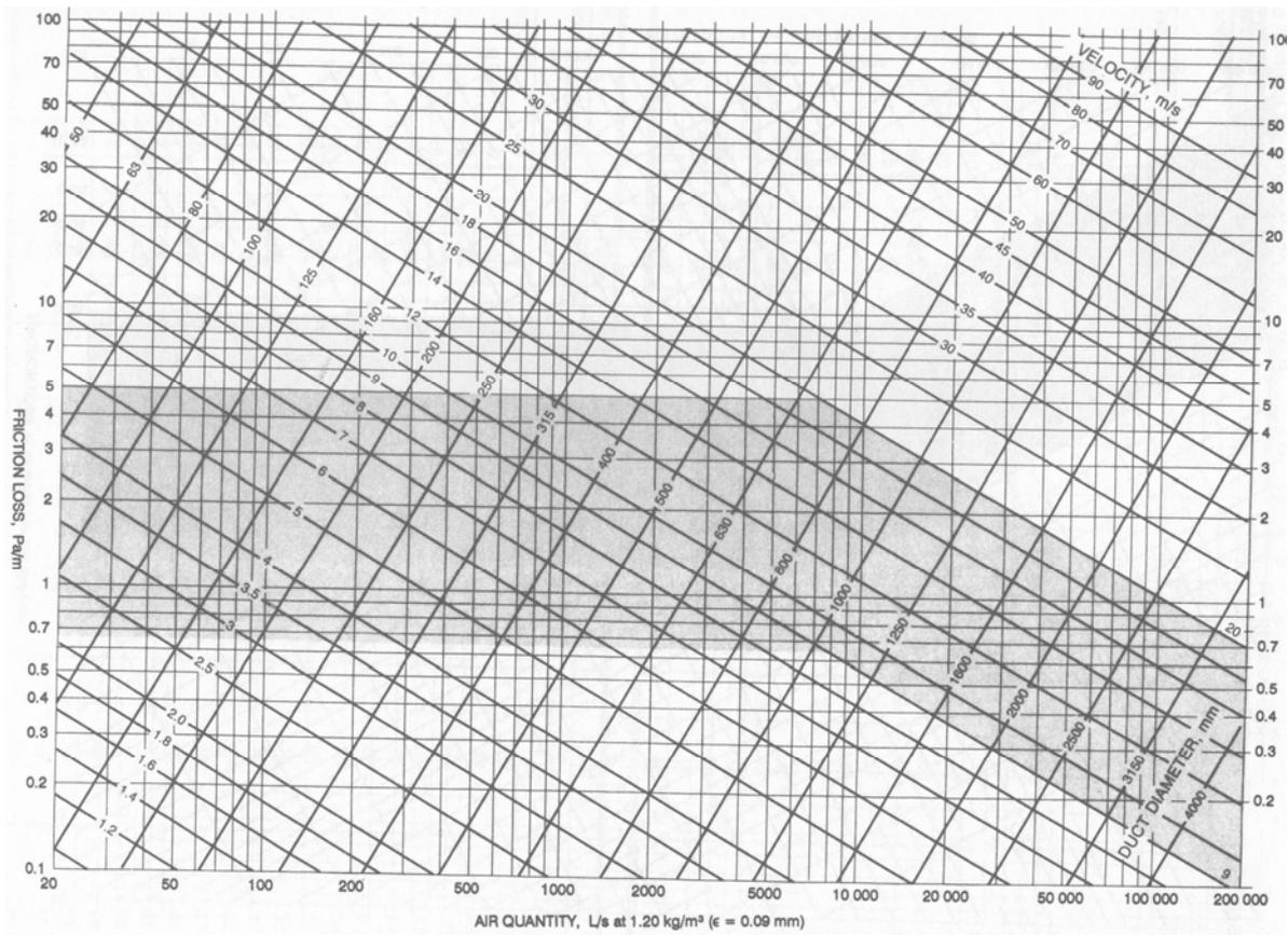
**Fig. 1c Straight duct friction losses**
