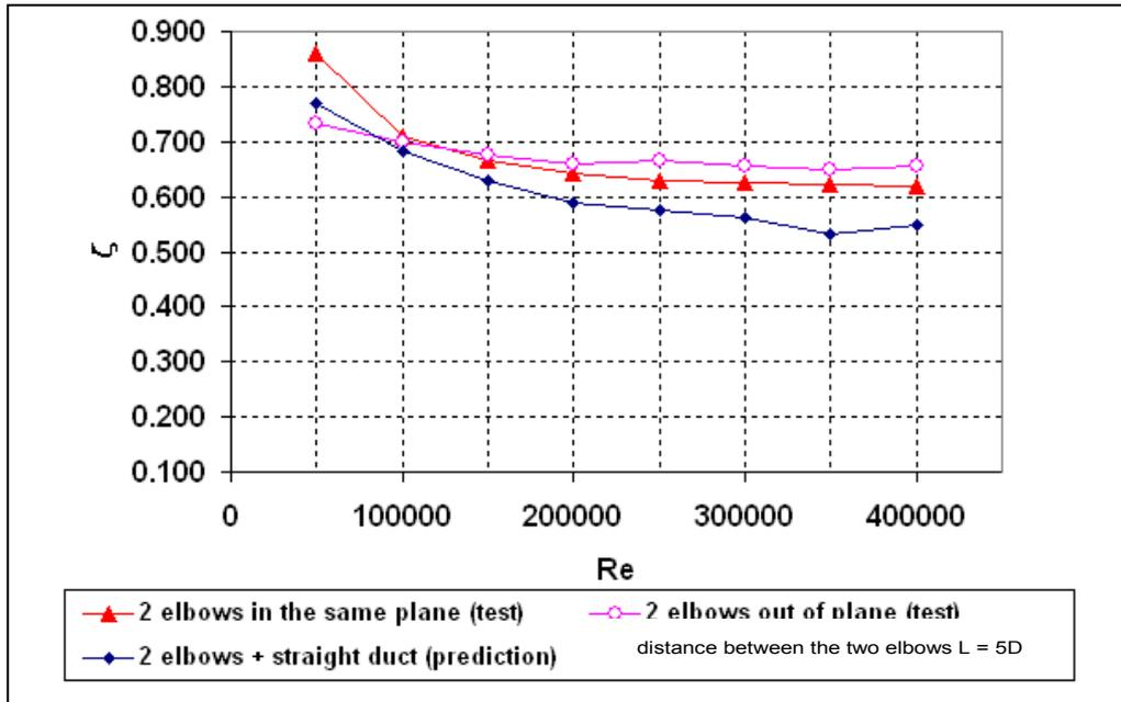
Fig. 8 Energy loss coefficient of 2 elbows separated by a duct  $L/D = 5$
