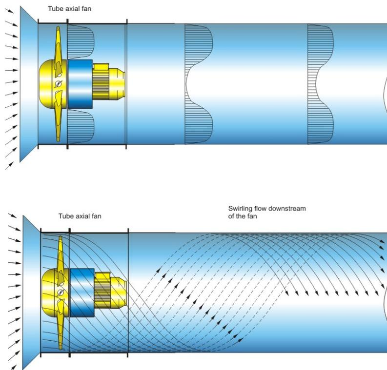
**Fig. 14 Tube Axial Fan showing distorted velocity profile and Swirling flow downstream**
