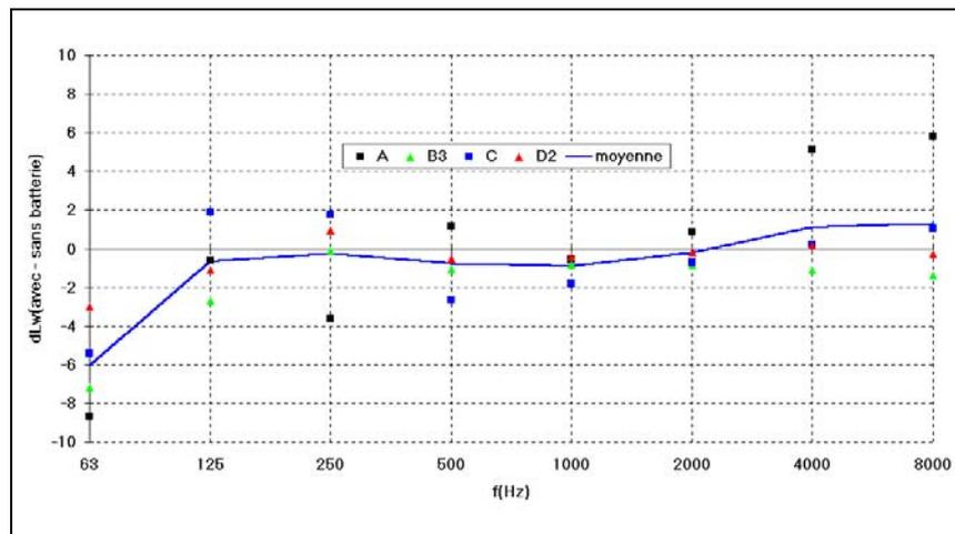
**Fig. 26 Exchanger at the fan discharge**  $dL_W \text{ (dB)} = L_W \text{ with exchanger} - L_W \text{ without exchanger}$
