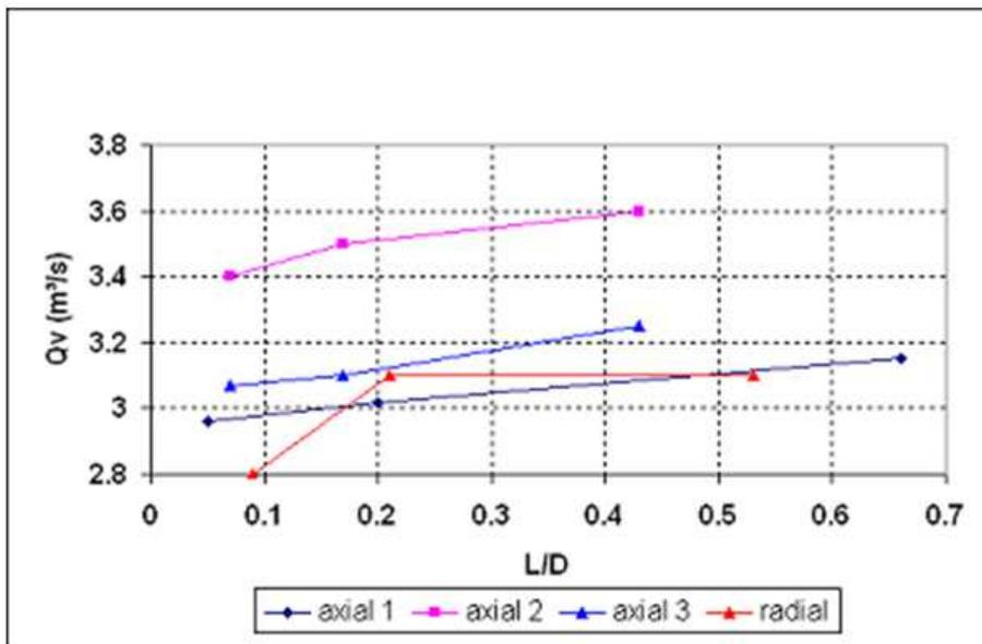
Fig. 27 Influence of the distance between the fan and the radiator on the airflow
