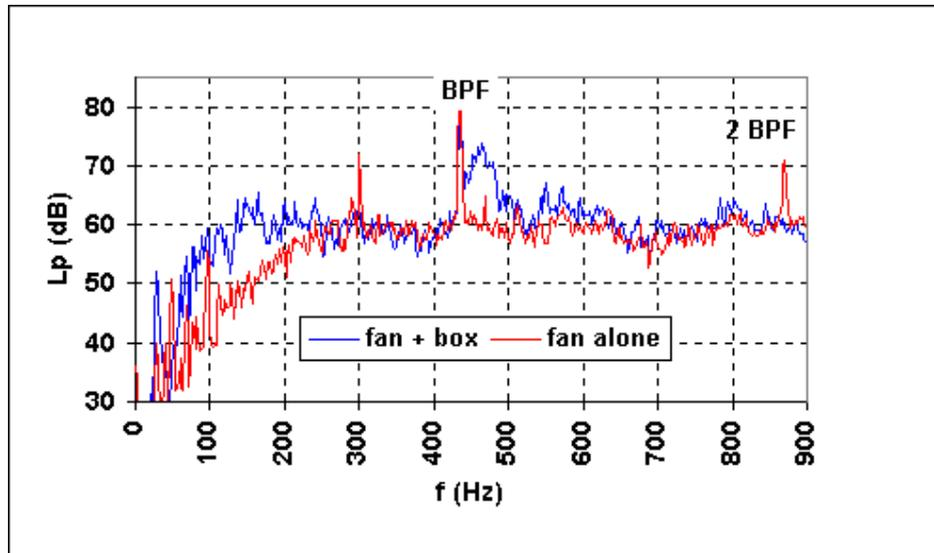
**Fig. 20** Narrow band sound pressure spectra measured with and without the inlet box
