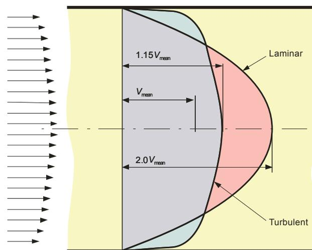
Fig. 2: Laminar and turbulent velocity profiles
