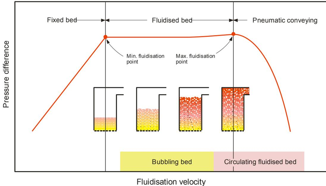
**Fig. A2 Pressure loss in the flow through bulk material**
