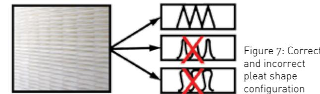
Figure 7: Correct and incorrect pleat shape configuration
