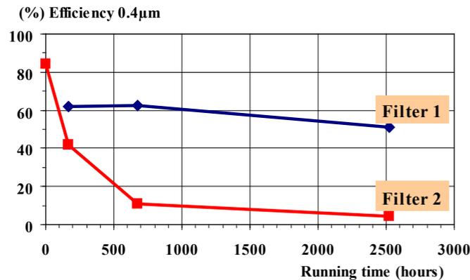
Figure 3: Increase of efficiency due to electrostatic charge
