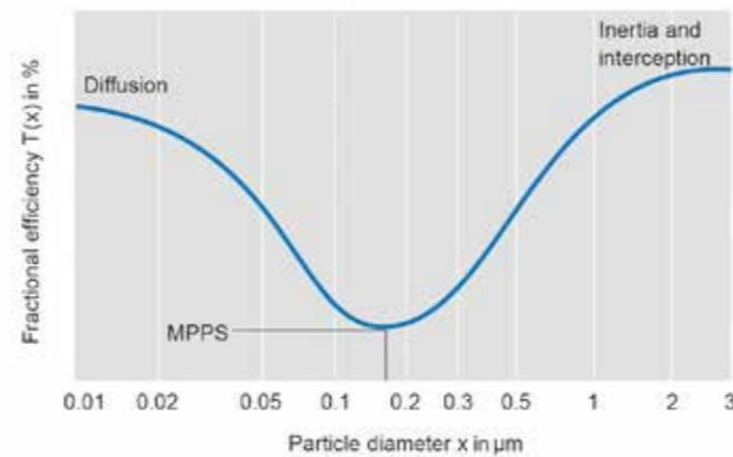
Figure 4: Transport mechanisms in particle separation on fibres
