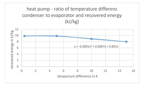
The two systems combined as one heat recovery system then show the following behaviour.
