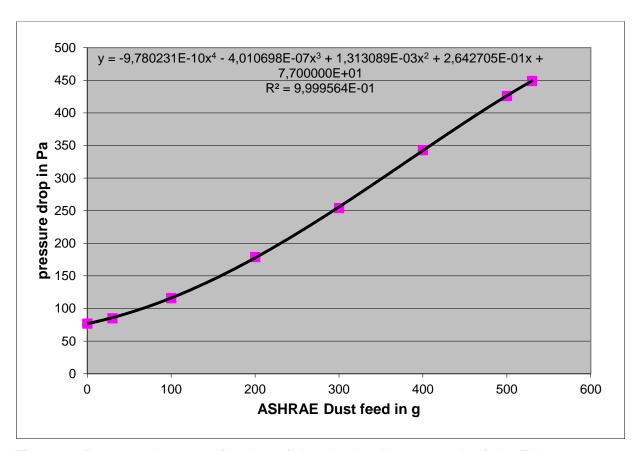
**Figure 1**: Pressure drop as a function of the dust loading as result of the EN 779 test at 0.944 m<sup>3</sup>/s. The function plotted on the top of the diagram shows the parameters a, b, c and d of Eq. (2) resulting from a curve fit of a polynomial of 4<sup>th</sup> order to the test data and the related coefficient of determination  $R^2$ .
